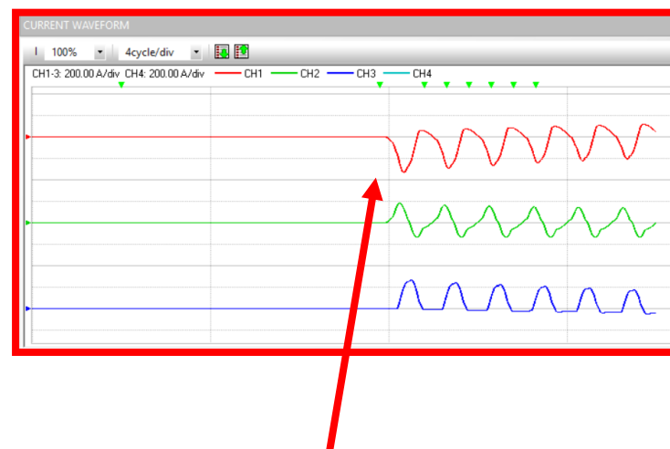
Figure 14: Inrush Current of unusual transformer TR2, which noticed the steady current of phase R and S.
