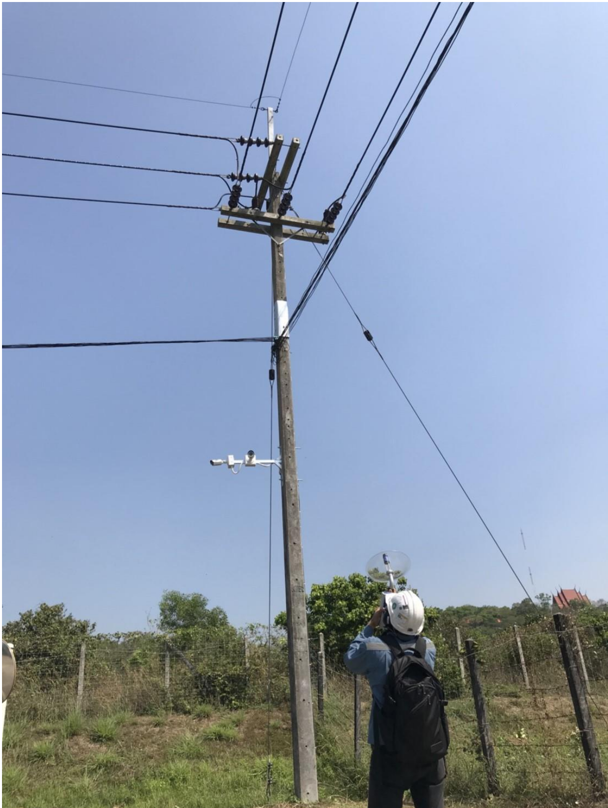
PD TEST BY ULTRADISH MODE AT 22 kV DISTRIBUTION LINE 19
