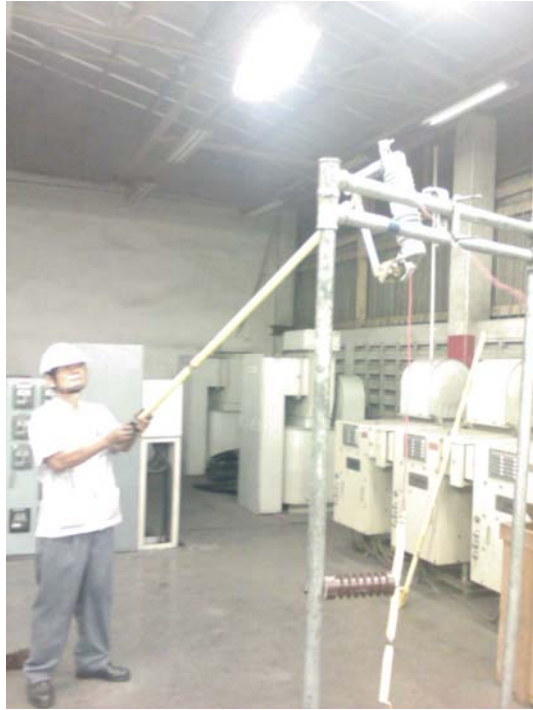
FIG.1 GROUND FAULT SIMULATION
