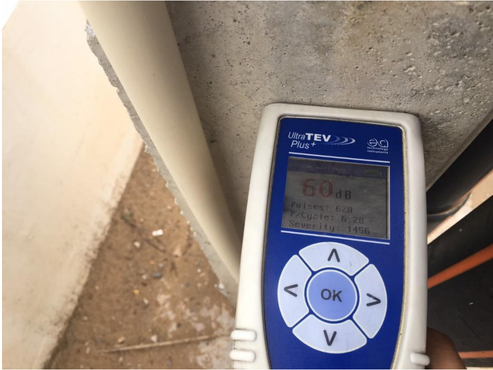
PARTIAL DISCHARGE DETECTED METHOD BY TEV MODE
