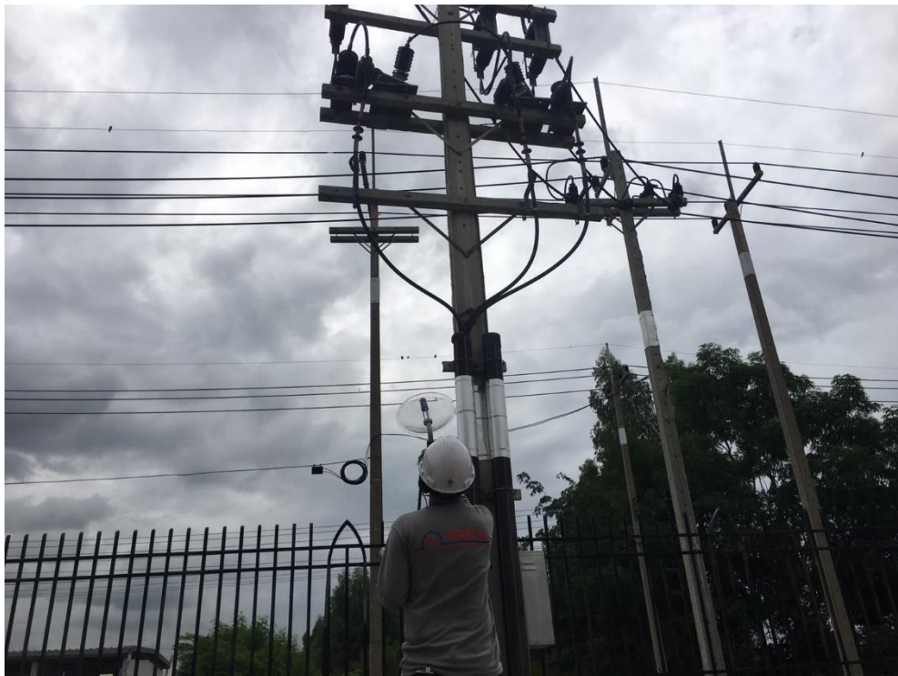
PARTIAL DISCHARGE DETECTED METHOD BY ULTRADISH MODE
